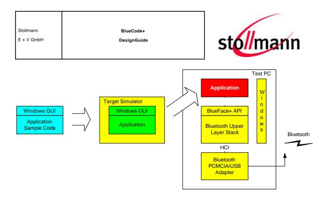
In a second step the application and the Bluetooth Upper Layer Stack will be integrated on the embedded system according to the previous chapter.
