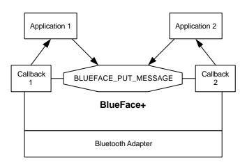
The BlueFace+ messages contain data and signaling information, covering all types of message exchange between the application and the Bluetooth stack. No additional API is required.
