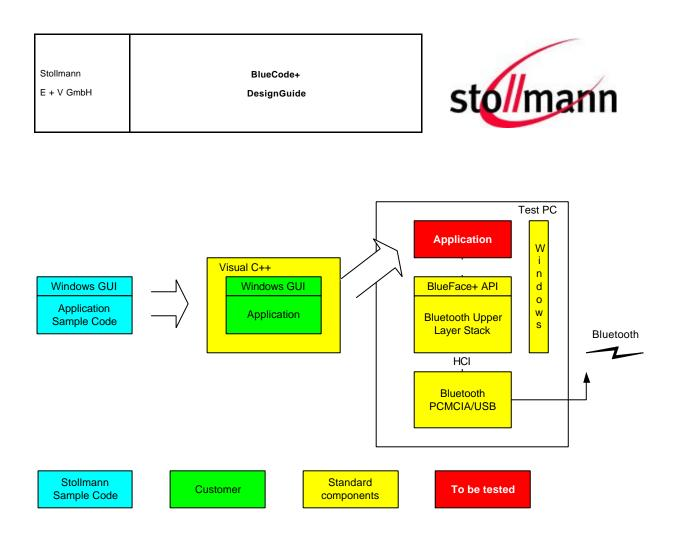
The sample code may be compiled to test it on a Windows system. It can then be modified for customer specific applications.
